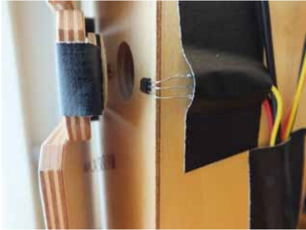
Figure 1: This picture shows a magnet which is under the tape on the key, and the magnetic field sensor on the instrument's body. © Simone Conforti
