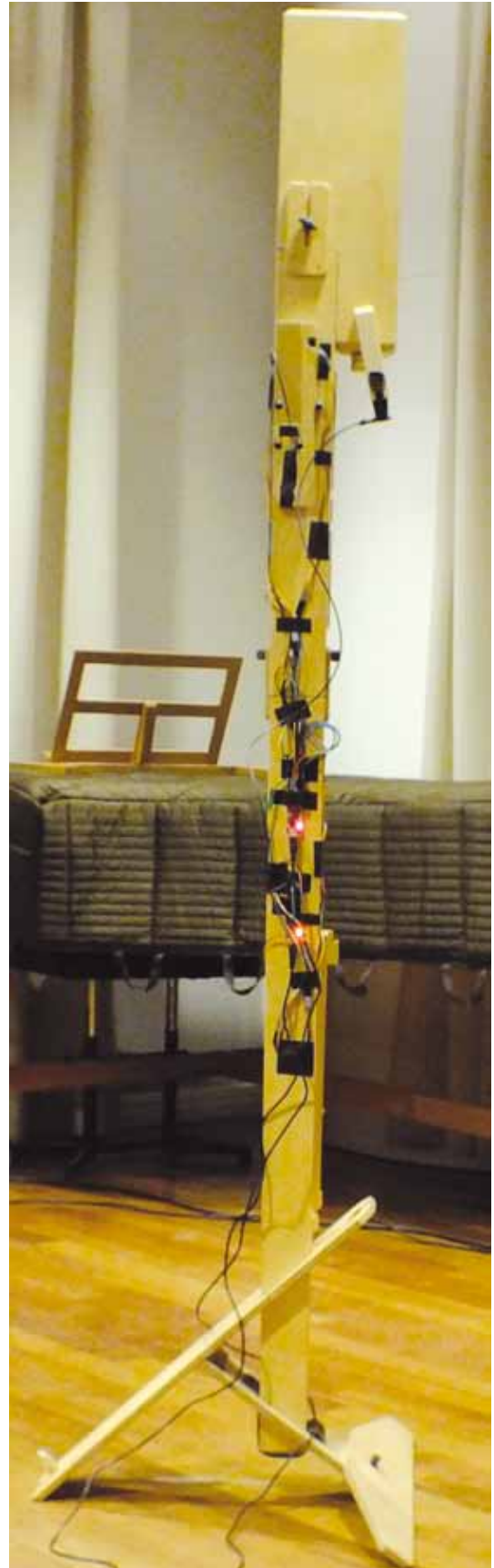
Figure 2: Paetzold recorder fully equipped with sensors. © Simone Conforti
